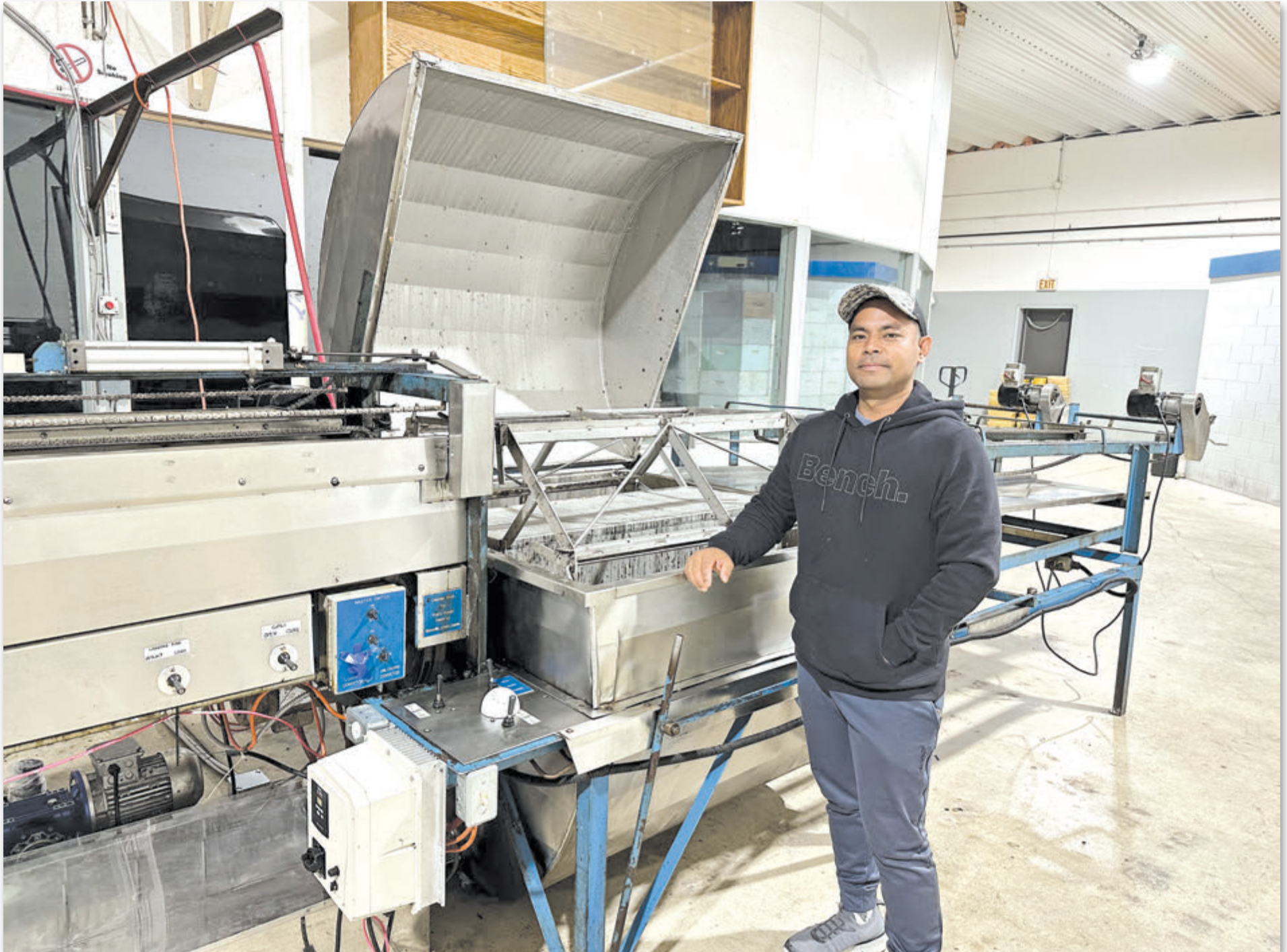
Jeffrey Mangubat shows off the large extractor, used for spinning frames to release honey.
